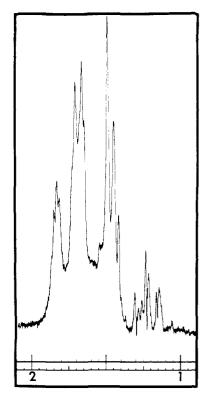
Figure 1. The 100-MHz nmr spectrum of VI; solvent CCl<sub>4</sub>,  $\delta$  in ppm from tetramethylsilane.
